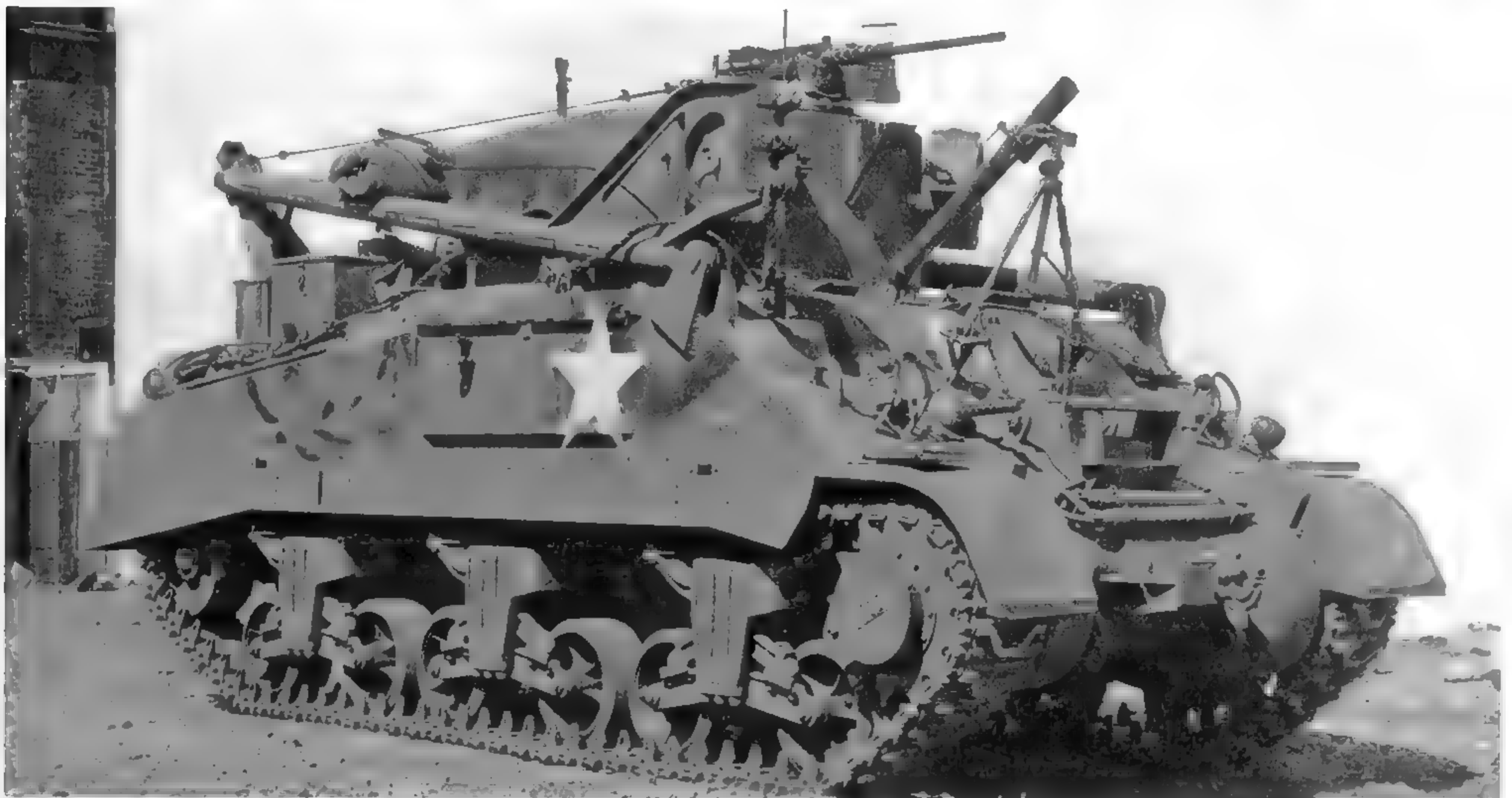
The M32B3 was based on the Army's standard welded-hull M4A3 Sherman tank. It carried the same equipment as the M32B1, although the difference in hull shape required that the stowage be laid out differently. (U.S. Army photo)
